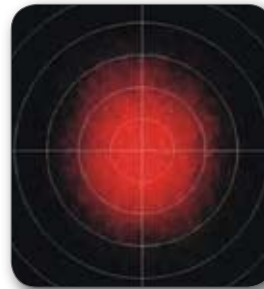
Standard diffuse material: laser reflects but scatters
